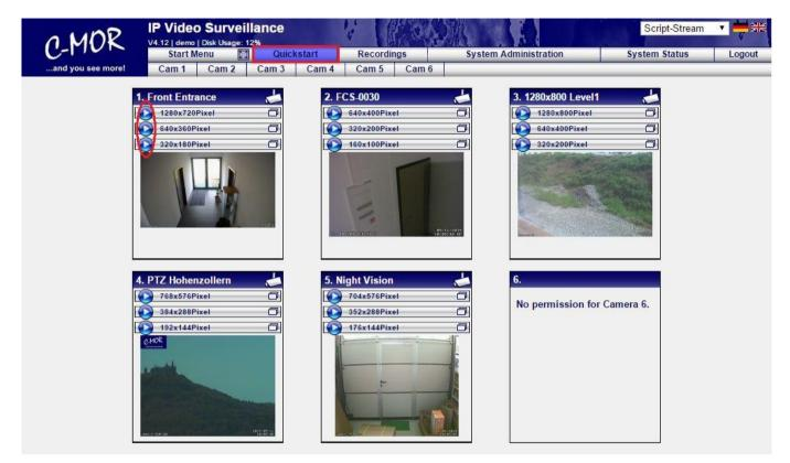
The Quick Start Page has a great advantage! It starts up quickly even it is accessed through a slow Internet connection. The small thumb nail camera pictures are updated in a high refresh rate only. This means that this page is not usable for live monitoring.
